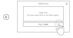
FILL TANK to flush the tank
