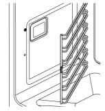
Slide the rear tabs of the side rack back onto the mounting studs, ensuring the rack is firmly pushed up against the side wall of the oven.
