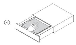
Before pressing the play button  $\triangleright$ , hold down the lid so the gasket forms a seal with the product.
